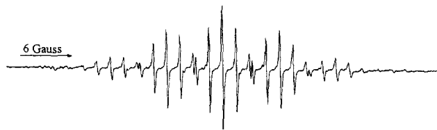
Fig. 2. EPR spectrum obtained by addition of silyl radicals generated by hydrogen abstraction from polysilane 2 with duroquinone.
